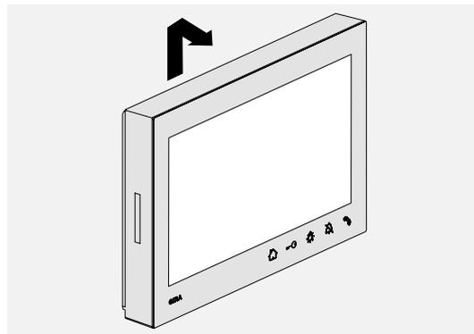
To remove the home station, support the sides and push firmly upwards with your thumbs until it is released by the catch mechanism.
