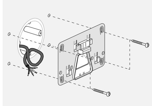
The home station's mounting plate should be fixed centrally over the cable outlet.
