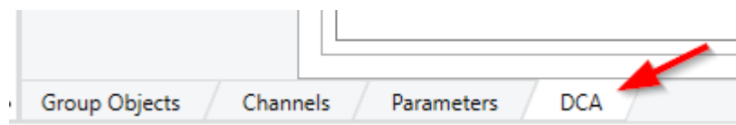
Figure 59: DCA tab in the configuration window for calling up the Device Configuration App
