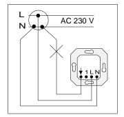
Relay Contact Insert Connection Using the Simulation Switch **Attachment**
