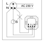
Disconnect the relay contact insert via switch 'S'.
