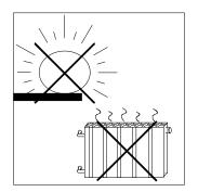
Avoid interference sources e.g. lamps or heaters within the detection range of automatic switches.
