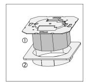
In order to guarantee protective system IP 44 for water-protected units, sealing flange @ must be installed into the flush-type box together with insert @.
