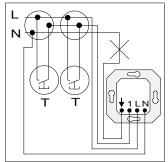
Existing two-way switches can be replaced by T push-button switches (normally open contacts).
