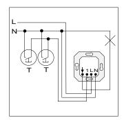
If the relay contact insert is combined with the simulation switch attachment, and if mechanical extension push-button switches (T) are to be connected, use the schematic diagram shown on the left.
