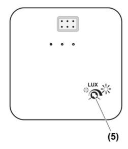
Figure 2: Back of cover: Adjuster for brightness threshold
