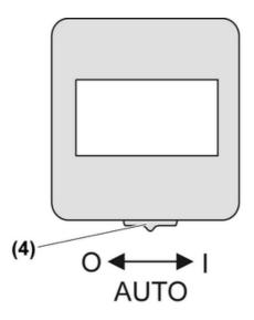
Figure 4: Operating mode switch
