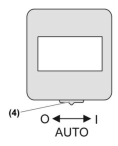
Figure 3: Operating mode switch
