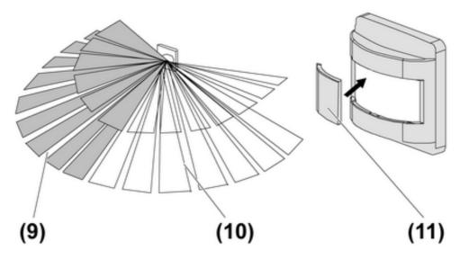
Figure 10: Using a cover plate
