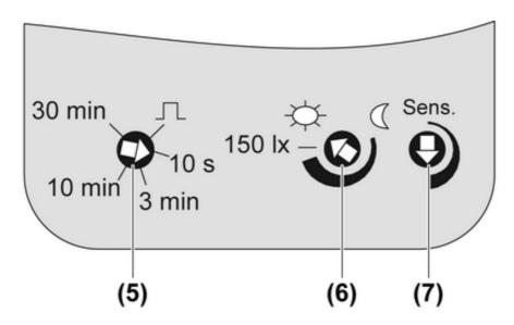
Figure 9: Adjusters on the rear
