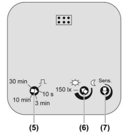
Figure 2: Adjusters on the rear
