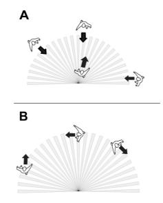
Figure 7: Detection area dependent on the direction of movement
