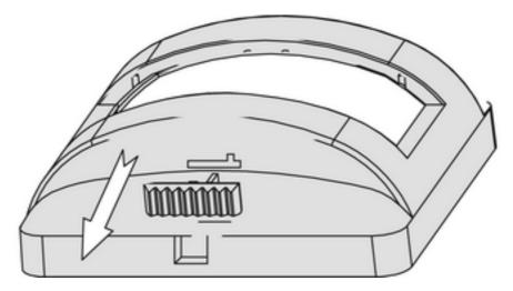
Figure 5: Removing the operating mode switch
