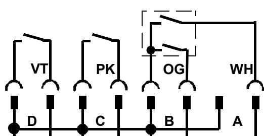
The black-white cable cores from a mutual reference potential in order to be able to connect switches for series or venetian blind (see fig. below).
