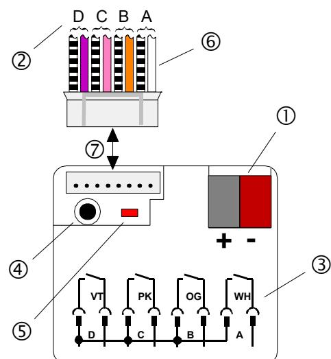
Programming the physical address is being undertaken by means of the programm key ④ and the program LED ⑤.
