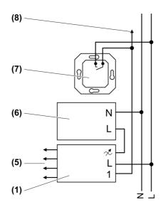
Figure 2: Connection diagram
