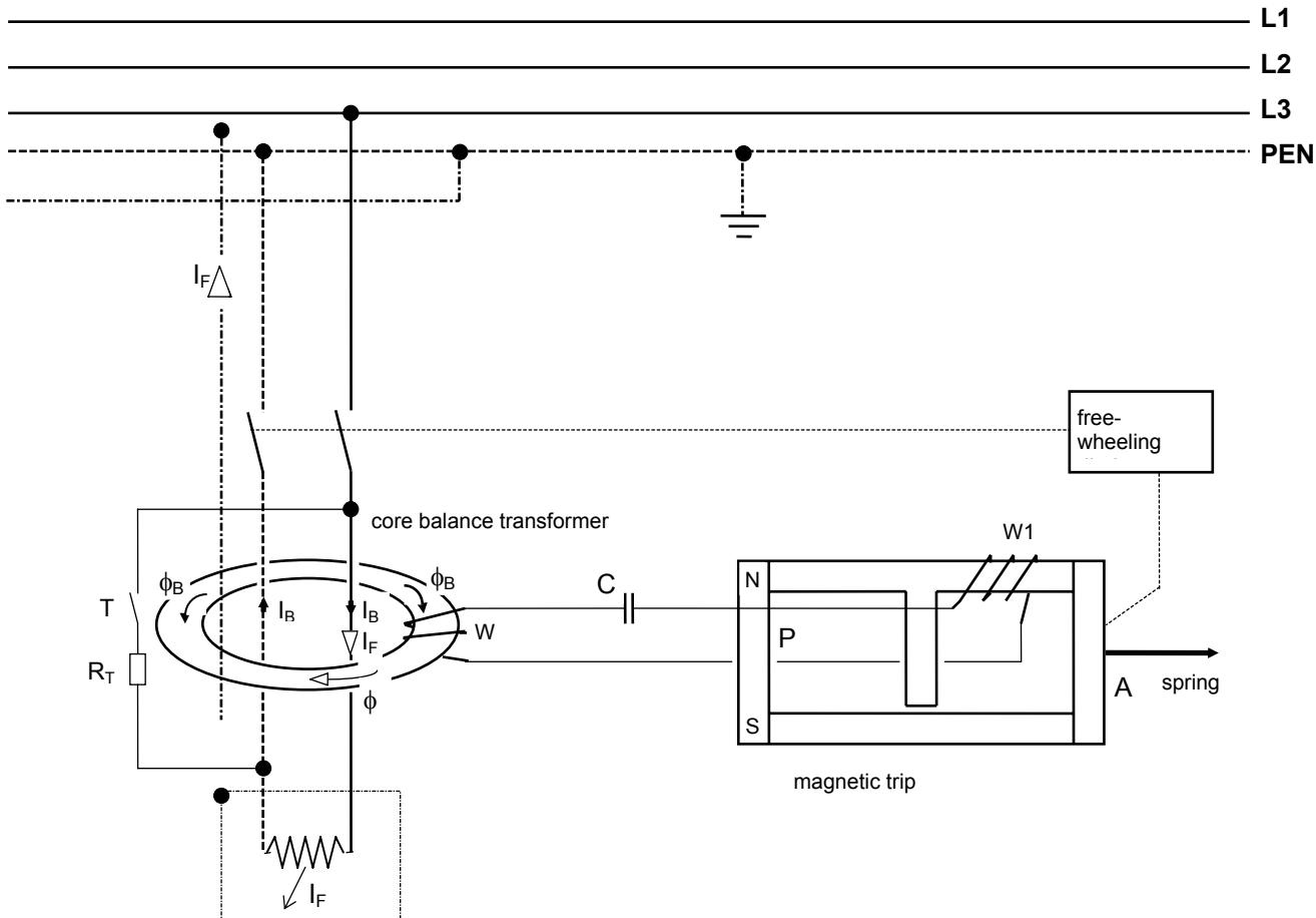
In the case of a fault, i.e. if a fault current  $I_F$  leaks to earth, and additional magnetic field  $\phi_F$  is generated, inducing an AC current in the trip winding W of the core balance transformer which is fed to the magnetic trip.
