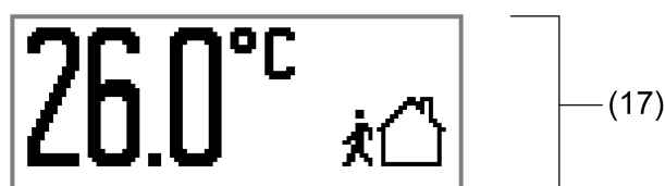
picture 51: Example of a basic display with one display area (Room temperature, operating mode display)
