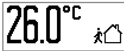
picture 7: Example of a basic display with one display area (Room temperature, operating mode display)
